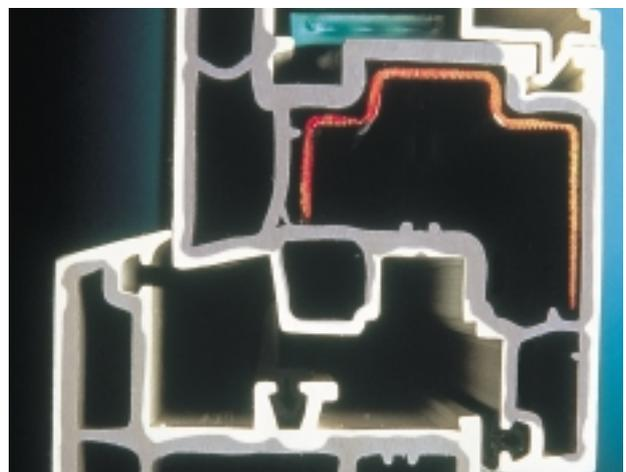
*Cross section of a PVC-U window frame using 70% recycle*
